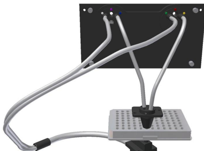
Figure 18: Principle drawing of top and bottom optics
