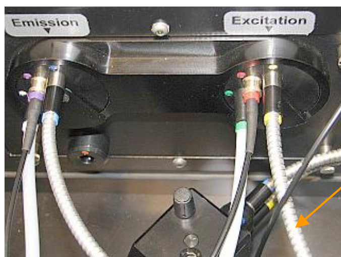
Fig. 23 Final look of the installed TRF optic head and light guides.
