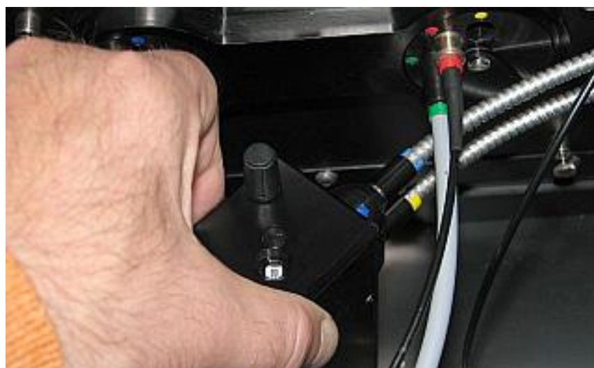
Fig. 21 Turn the TRF optic head 45 degrees
