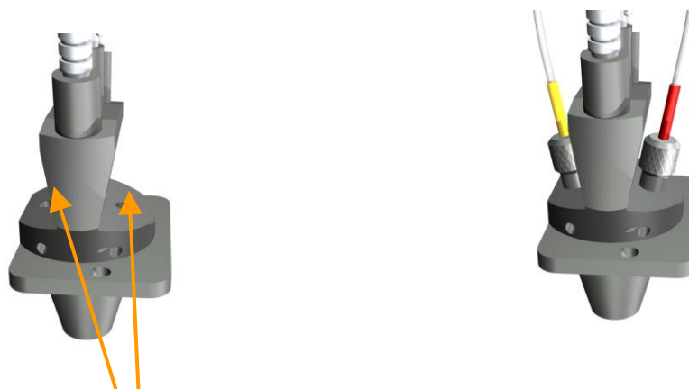
Figure 15: Holes to position reagent needles in the measurement head
